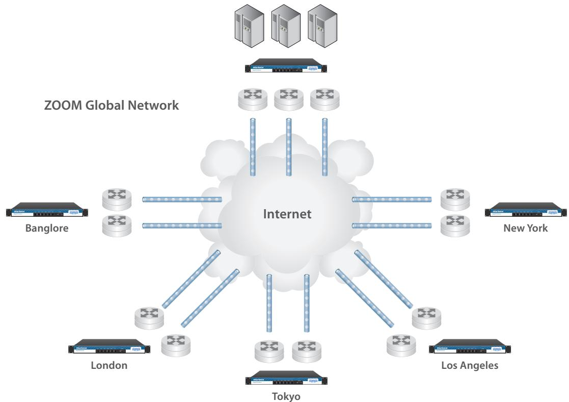
**Private Cloud Fully Meshed Redundancy:** With our Private Cloud tunnels a network administrator can configure a completely redundant and fully meshed remote office solution. Full meshing means that even in the event that two simultaneous network outages occur at both ends of the tunnels, that the remote sites stay up and running.
