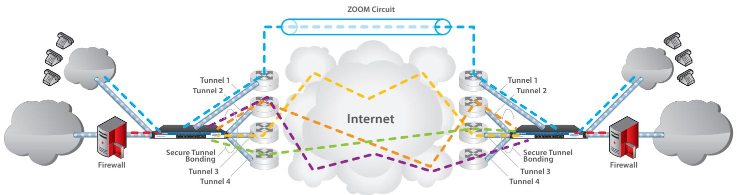
**Private Cloud Best Path Routing:** Built-in to the routing mechanism for our Private Cloud tunnels is our Best Path Routing technology. Best Path Routing uses network thresholds to determine which tunnel path is the best one to use for sending each new session. This ability ensure that even when a link begin to perform badly that the Private Cloud tunnels are always leveraging the best possible connectivity provided via the available WAN links.
