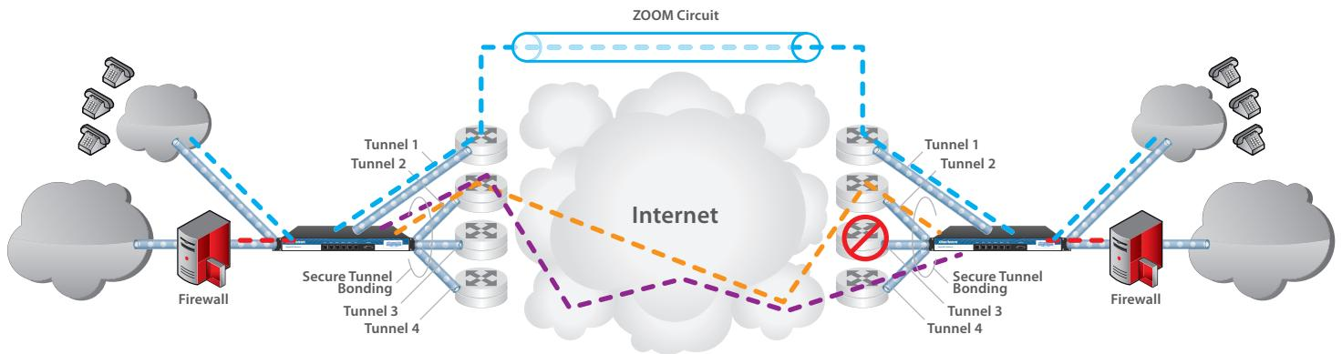
**Private Cloud QoS:** As packets traverse the Private Cloud tunnels, packet labeling is performed (as in ZOOM networks) with the label state remaining constant from end-to-end. This ToS/Diffserv labeling can be used to classify packets based on application type in order to prioritize critical applications. In addition, the EdgeXOS platform incorporate full rate-shaping and bandwidth partitioning at each end of the tunnel thus guaranteeing critical application priority between sites.
